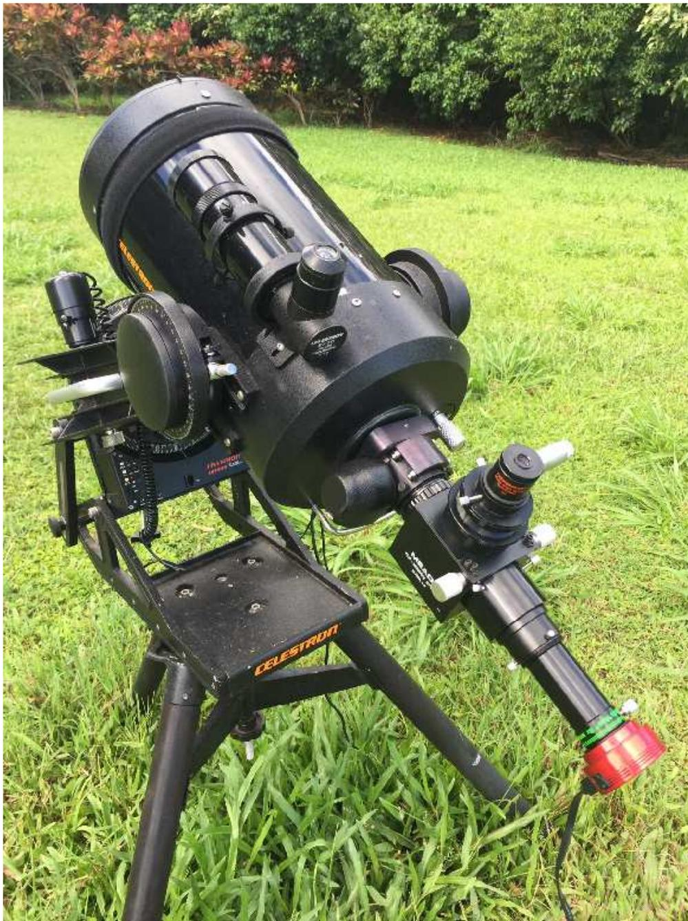
Figure 1: The 8-inch (200-mm) SCT telescope with 3x Barlow lens attached and ZWO ASI CMOS camera
