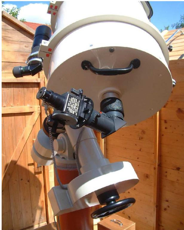
Figure 2: 325-mm/f19 Cassegrain running on Alt 7AD equatorial mount with MECA PRECIS Double Image Micrometer
