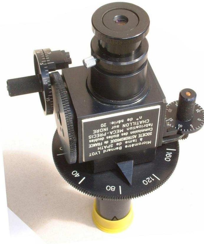
Figure 3: The MECA PRECIS Double Image Micrometer ‘Bernard Lyot’, here with a 10 mm Zeiss ortho eyepiece. At right: screw for PA setting: rotates the box around the angular scale. At left: screw for distance setting: rotates the calcite plate located under the eyepiece. A setting of  $\pm 10$  corresponds to a distance of  $0''.83$ .
